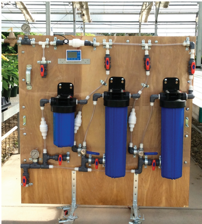
Figure 3. A research-sized GAC filtration system being tested at the University of Florida. Multiple filters can be turned on or off to vary the filtration level.
